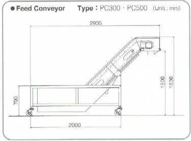
\* PC300 and PC500 are 300mm and 500mm in conveyor belt's width respectively.
